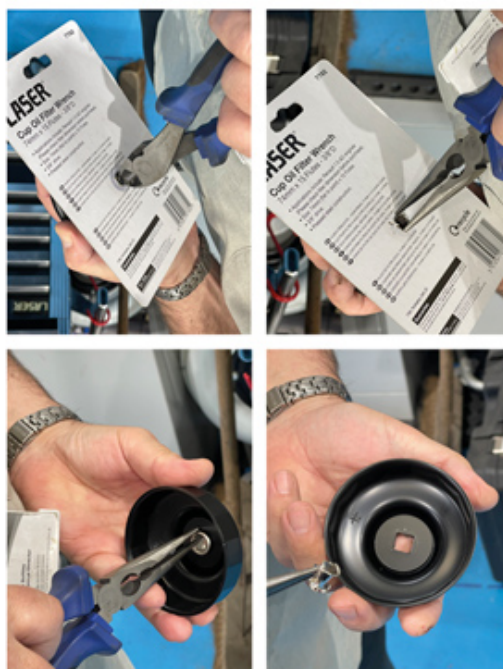
Brass rivet is used to hold backing card only, remove rivet before use.
